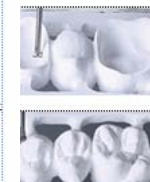
Milling Bur 1,5 A Used to mill pre-sintered zirconia (abutment)
